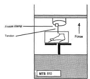
Fig. 1: The tendon is attached to the testing ram of the material testing system though a freeze clamp. The cadaver specimen is anchored to the system base through smooth wires placed in the calcaneus and first metatarsal.
