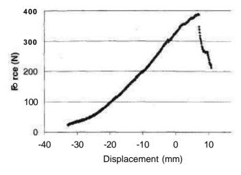
Fig. 2: Load displacement curve for tendon to tendon fixation.
