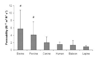
FIGURE 6. Comparison of the permeability (femoral and tibial sides combined) at the central location in the six tested animal models. Data shown as mean  $\pm$  standard deviation. (#) indicates a significant difference between either the bovine or porcine permeability and the canine, human, baboon, or lapine permeability (p < 0.02).
