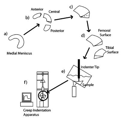
FIGURE 2. A schematic diagram of the testing procedure. The medial meniscus (a) is separated into anterior, central, and posterior regions (b). The meniscus is split in the transverse plane (c) and separated so that the femoral and tibial surfaces can be tested (d). The meniscal sample is then attached to the sample mount (e) and tested in the creep indentation apparatus (f).
